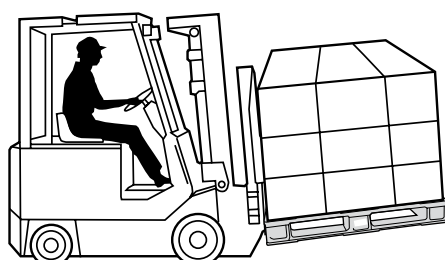
Dynamic load Max Uniformly distributed load that a pallet can carry when transported by forklift.
