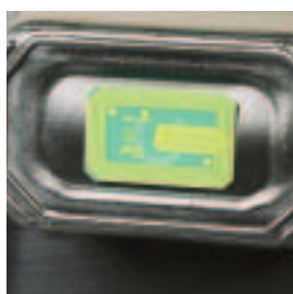
Imbedded RF-tags in the skids assure traceability.
