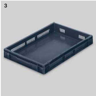
3 12 litres - Ref. 21015 polypropylene solid base, ventilated sides Ext. dim.: L 600 X w 400 X h 73 mm Ext. dim.: L 23.6 X w 15.8 X h 2.9" Int. dim.: L 555 X w 355 X h 62 mm Int. dim.: L 21.9 X w 14.0 X h 2.4" Wt: 1.02 kg/2.2 lbs., Colour: grey . SKU quantity: 85
