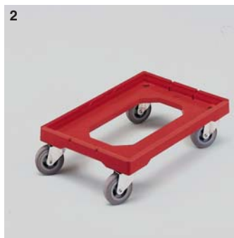
2 Ref. 91011 minimum order item Rubber wheels on galvanised mountings Dim.: L 604 X w 402 X h 162 mm Dim.: L 23.8 X w 15.8 X h 6.4" four swivel castors, Ø 100 mm/4" loading: 250 kg/550 lbs Wt: 4.00 kg/8.8 lbs. Colour: red.
