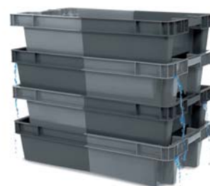
Colour: grey/light grey 3 38 litres – Ref. 12041* with external drainage Ext. dim.: L 800 x w 450 x h 190mm Ext. dim.: L 31.5 x w 17.7 x h 7.5" Int. dim.: L 624 x w 372 x h 155mm Int. dim.: L 24.6 x w 14.6 x h 6.1" nested height: 55mm / 2.2" Wt: 2.60 Kg/5.7 lbs.
