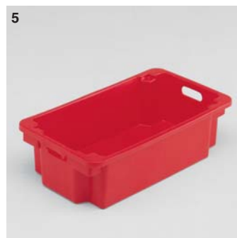
5 44 litres - Ref. 11044 Ext. dim.: L 755 X w 435 X h 190 mm Ext. dim.: L 29.7 X w 17.1 X h 7.5" Int. dim.: L 680 X w 360 X h 170 mm Int. dim.: L 26.8 X w 14.2 X h 6.7" nested height: 58 mm/2.3" Wt: 2.25 kg/5.0 lbs., Colour: white, red. SKU quantity: 51
