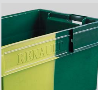
Embossed moulding in relief during manufacture.
