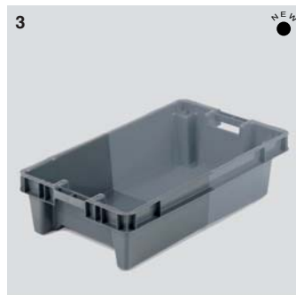
Colour: grey/light grey 3 38 litres – Ref. 12041* with external drainage Ext. dim.: L 800 x w 450 x h 190mm Ext. dim.: L 31.5 x w 17.7 x h 7.5" Int. dim.: L 624 x w 372 x h 155mm Int. dim.: L 24.6 x w 14.6 x h 6.1" nested height: 55mm / 2.2" Wt: 2.60 Kg/5.7 lbs.
