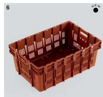
6 43 litres – Ref. AE215*** ventilated sides, drainage holes in base Ext. dim.: L 600 x w 400 x h 237mm Ext. dim.: L 23.6 x w 15.8 x h 9.3" Int. dim.: L 560 x w 360 x h 215mm Int. dim.: L 22.0 x w 14.2 x h 8.5" nested height: 69mm / 2.7" Wt: 2.00 Kg/4.4 lbs. Colour: brown-red
