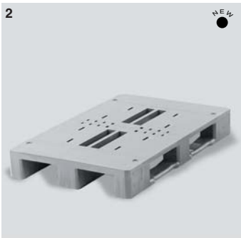
2 Ref. 3P300 pallet with 3 runners semi-solid deck Dim.: L 1,200 x w 800 x h 160mm Dim.: L 47.2 x w 31.5 x h 6.3" Wt: 21 Kg/46 lbs. Colour: light grey For use in temperatures from 0° to + 40°C
