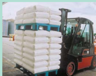
Stable block stacking.
