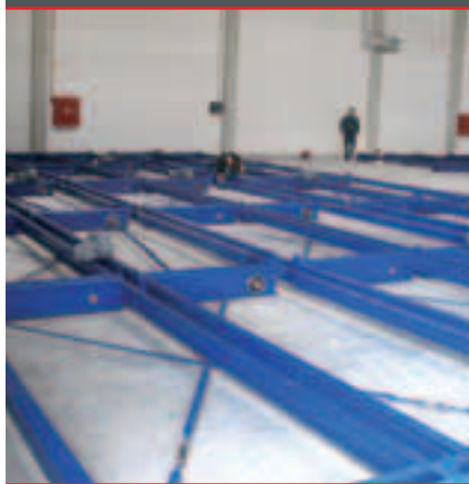
Drive elements for pallet- or cantilever racking
