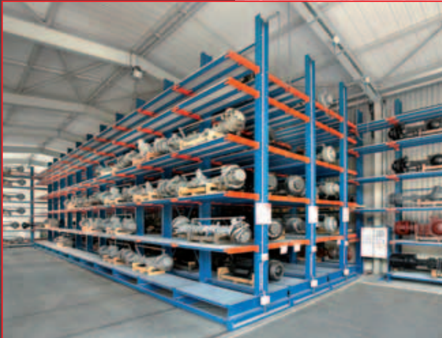
Cantilever racking equipped with metal mesh each level
