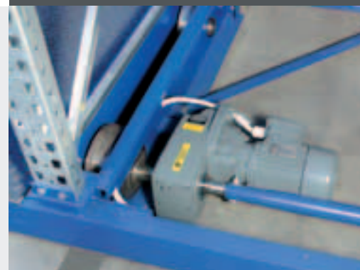
Detailed view on the maintenance free gear motor
