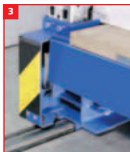
Light barrier in the aisle
