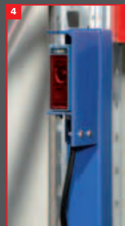
Light barrier in front of racking
