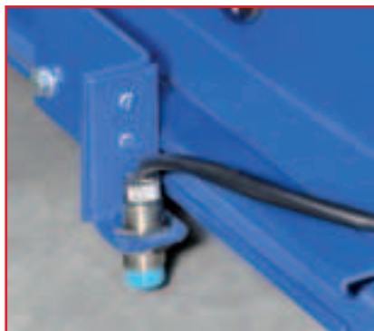
Magnetic switch at both outer drive elements
