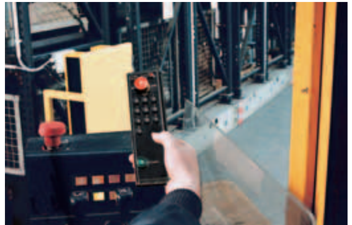
Operation with radio-control on the forklift: move the drive elements while drive towards the racking
