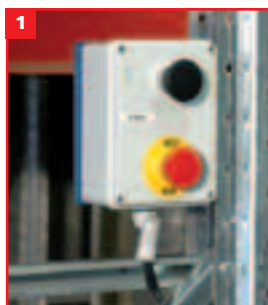
Emergency stop at each drive element
