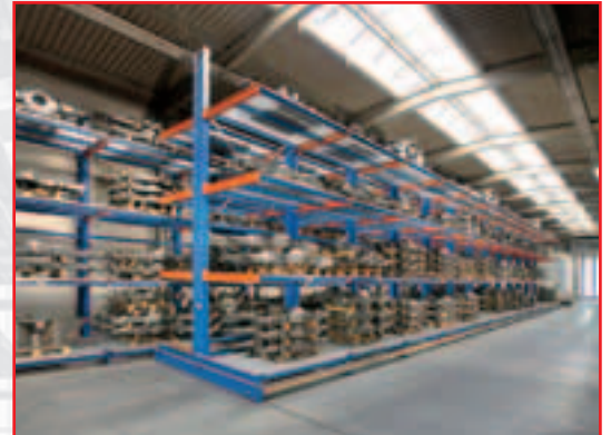
Cantilever racking equipped with metal mesh each level
