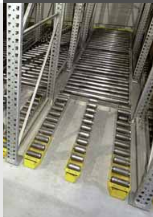
Bottom outlet divided into three parts
