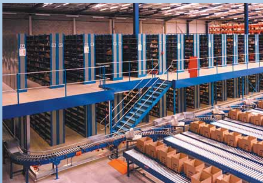
A QB2 multi-tier installation in an Engineering Distribution Centre.
