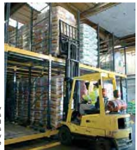
As pallets are picked a safety separator is activated. This holds the accumulated load of several tonnes and allows only one pallet to flow smoothly and securely to the front face.
