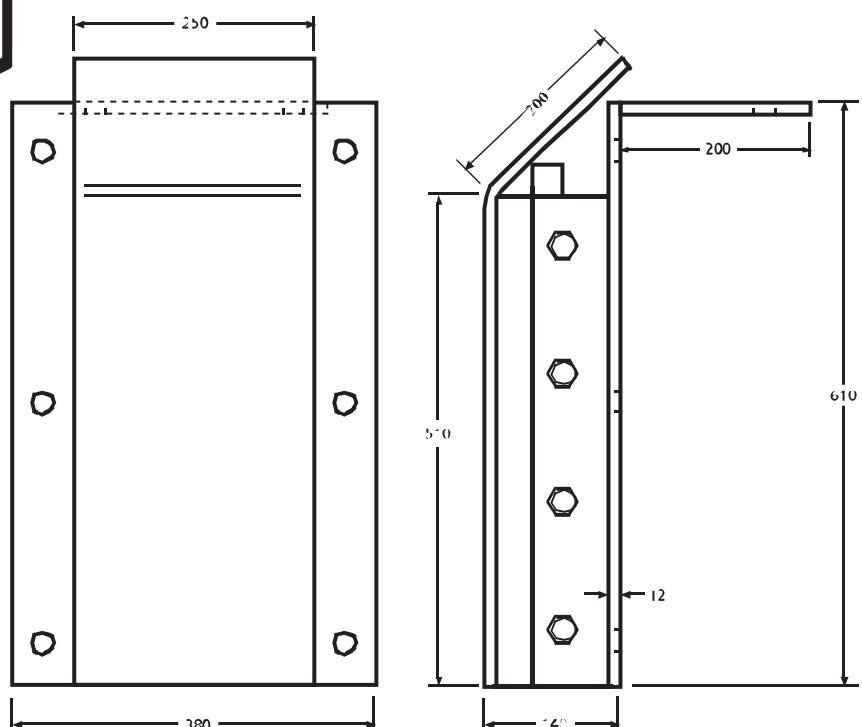
**STEELWORK FOR DOCK BUMPERS****HANDED DOCK BUMPER/PLATE ASSEMBLY****Part Numbers: SP/LH/FP750, DB/LH750, SP/LH/BP750****MATERIAL: STEEL & NATURAL/SBR RUBBER COMPOUND**
