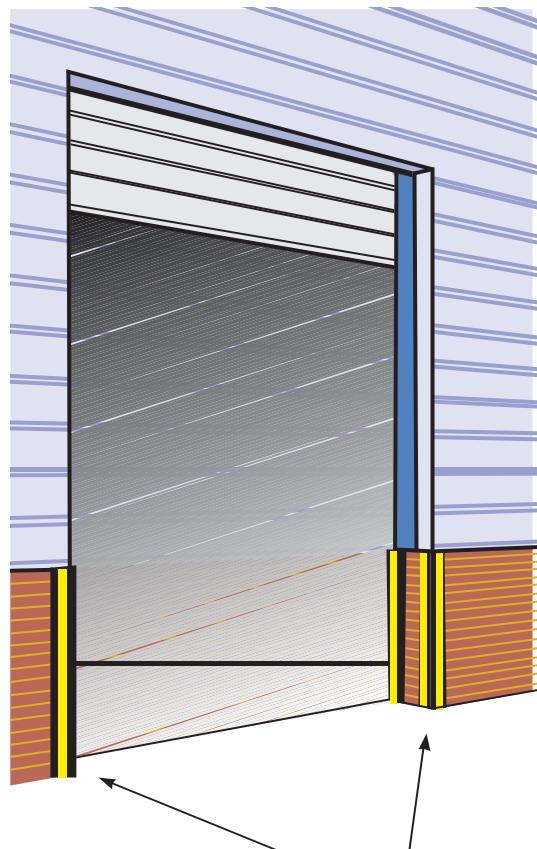
Typical usage protects any Brick or Blockwork corners from forklift damage
