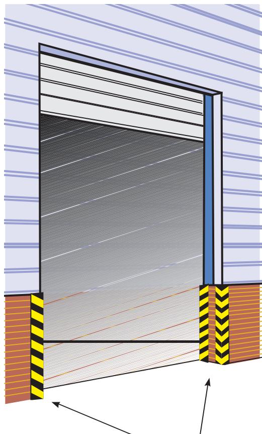
Typical usage protects any Brick or Blockwork corners from forklift damage
