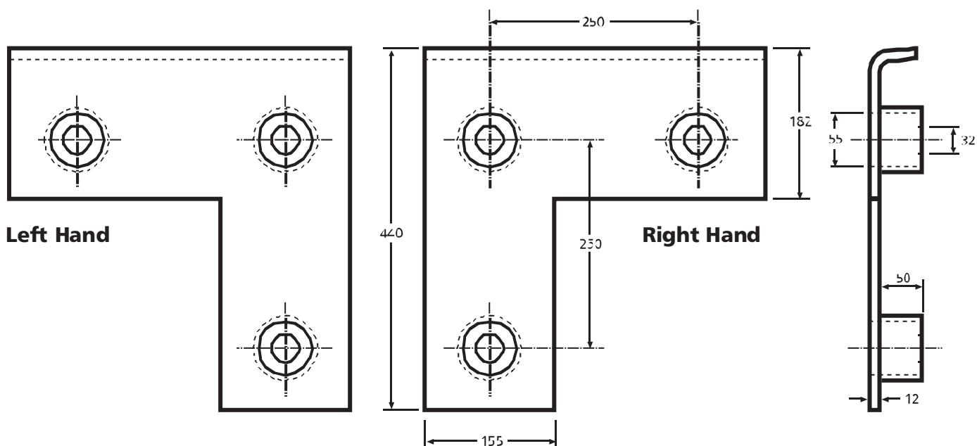
**Note:** - Plates are sold in pairs and are Left and Right Handed as shown.
