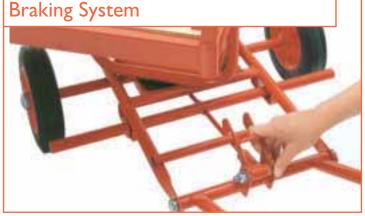
A clever simple to operate brake system, effective when the handle is in the upright position, finishes off the range of accessories but unlike the other options these are factory fitted and need to be specified at the time of ordering.
