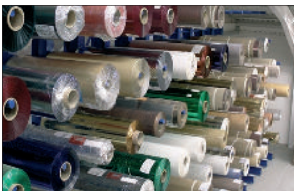
Cantilever rack with spindle arms to protect delicate rolls of material
